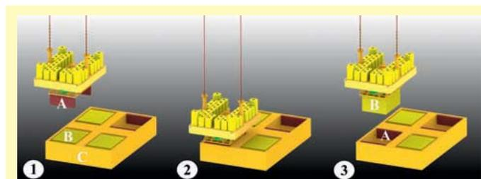
1. The SDV – c/w ballast weights (A) equivalent to the weight of the module (B) – is lowered to the foundation structure (C).
