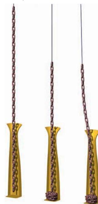
*Horizontal, vertical and rotational control by means of chains lowered into the SDV control chain towers, which behave as soft springs and minimise dynamic loading*
