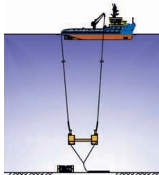
**Positioning of the SDV will be by means of two control chains suspended from the installation vessel and lowered into the chain towers**
